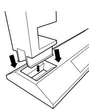
insert the wall frames into the slots on the base:
